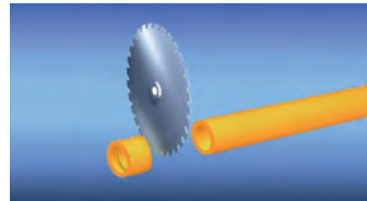
Cutting off the flange shoulder with hot saw (only for certain dimensions)
